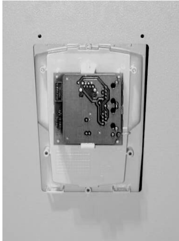
7. Insert the Panel Platform in the hole.
