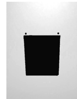
6. Take the mounting template and make a hole exactly the same size as the template on the door or wall for installation of the Panel Mounting Platform.
