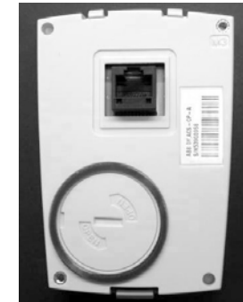
3. Place the Gasket around the Battery Compartment.
