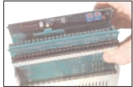
Figure 13. Pull the three-circuit board assembly from the housing.
