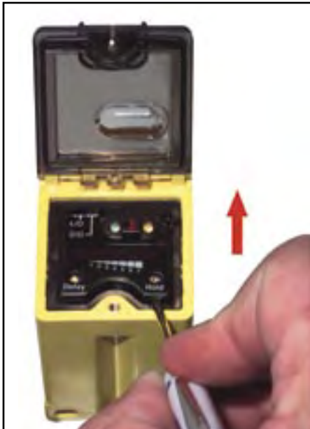
Figure 5. Insert a small screwdriver into the slot and lift the black cover to remove.
