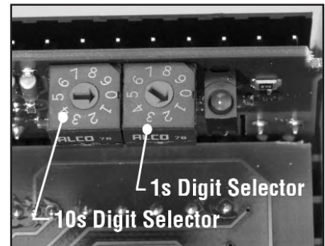
Figure 5. MAC ID address rotary selectors and LED
