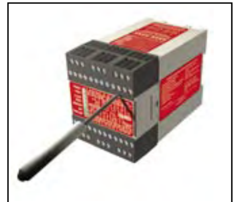
Figure 7. To remove the Module's terminal strips, insert a small screwdriver blade into each of the four slots at the top and bottom of the front cover.
