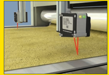
Dough Thickness Sensors measure the height of dough, adjusting the machine roller for thickness control
