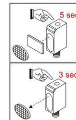
The sensor selects the best operating conditions according to the acquired points and adjusts itself in the DARK mode condition. The acquisition sequence has to be inverted to select the opposite operating modes.
