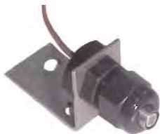
150062 & 836068 micro Thru-Fitting & MB-2 Mounting Bracket plastic fitting with lock nut, sealing nut, and hub 1.17" x 0.59" (29.7 x 14.99 mm) PG-7 thread
