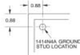
Ground stud location for 1414N4A
