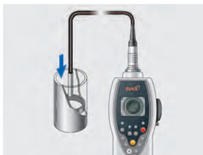
Inspection of the inside of metal parts
