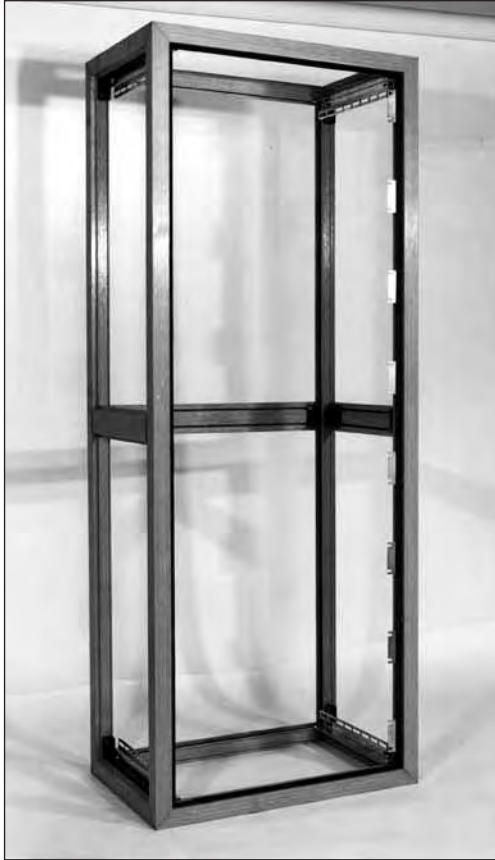
The framework is made up from pultruded sections of fiberglass (with 70% by weight of glass fiber). The corners are braced with interior fitted (and fully sealed) metal brackets. This gives an extremely strong and rigid structure.
