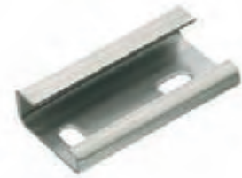
TS 32 mm according to EN 50035 (s = 1.5 mm)
