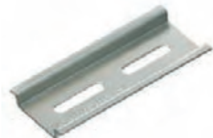
TS 15/5.5 mm according to EN 50045 (s = 1.0 mm)
