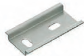
TS 35/7.5 mm according to EN 50022 (s = 1.0 mm)
